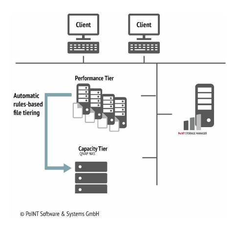
The town of Hof uses the software PoINT Storage Manager to automatically off-load inactive data.
