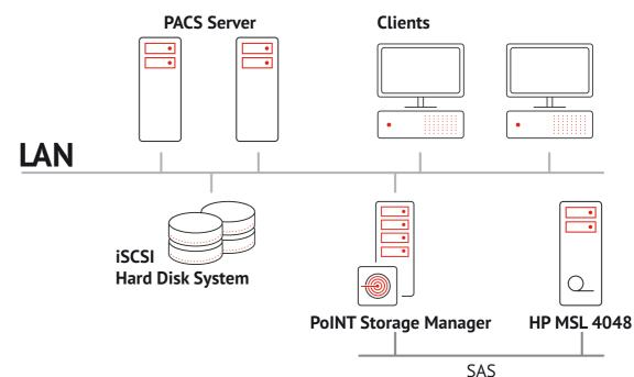
The hospital "DRK Krankenhaus Chemnitz-Rabenstein" was looking for a solution to archive old PACS data. Archiving should be carried out gradually on tape. In Tier 1 a hard disk system (iSCSI) was used for data to be archived and frequently accessed PACS data.
